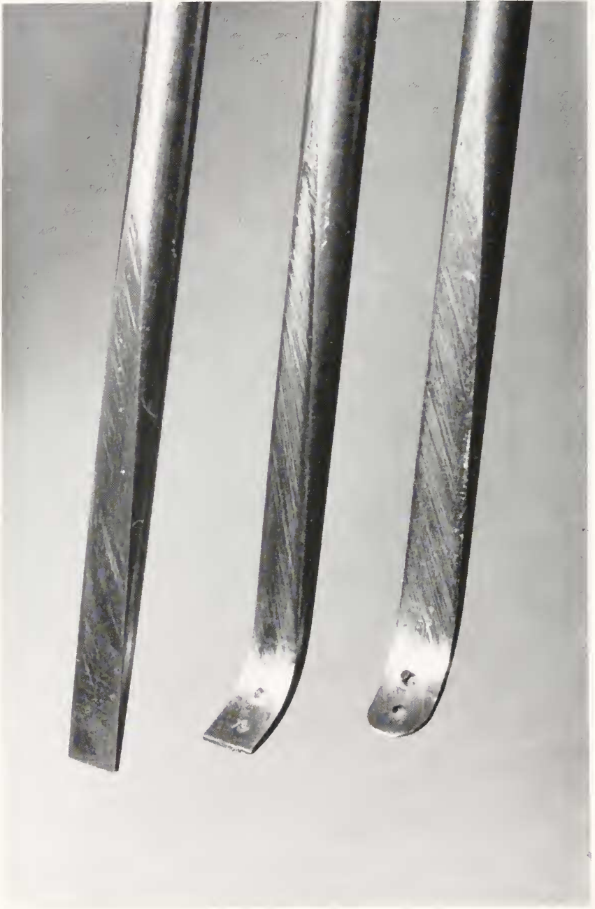
Figure 2. The three stages in making a raft spoon. Left to right: the taper has been filed; tip has been bent and punched; holes have been bored at punch marks and tip rounded.
